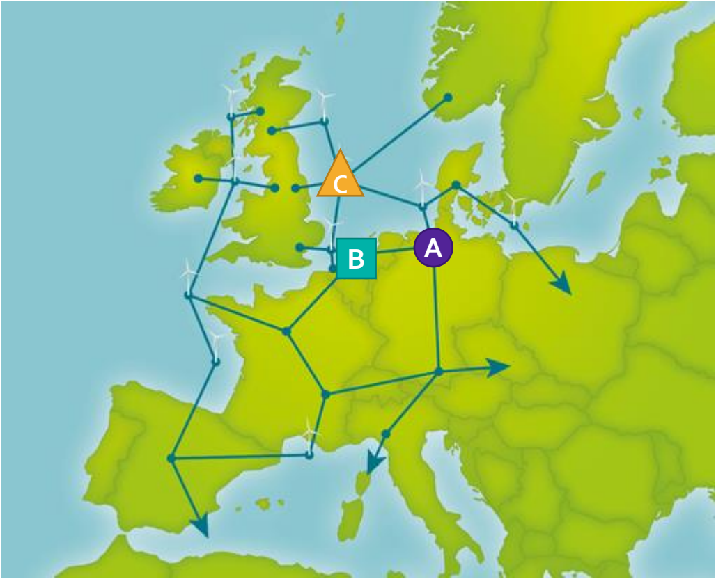
Multi-terminal multi-vendor HVDC system vision (Corbett, 2020)
